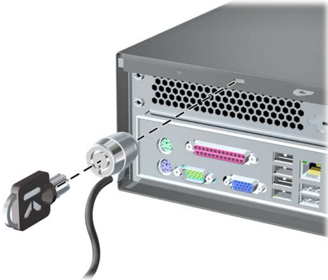
Figure 7-40 Installing a Cable Lock
